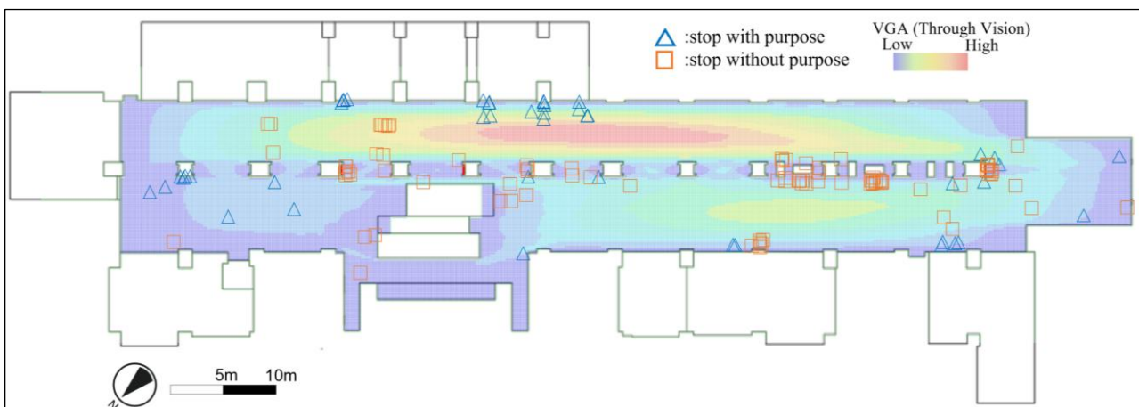
Fig.9 Pedestrian Locations and VGA (Through Vision) Results in the case of Kyobashi Edogrand
